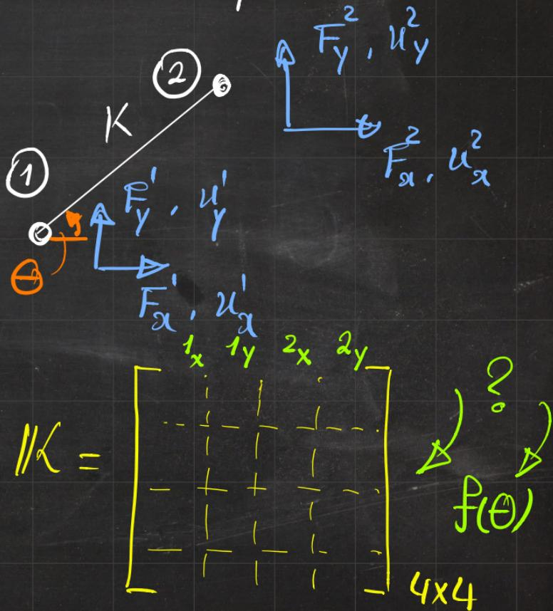
To compute stiffness of 1D element in 2D space
