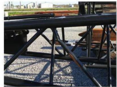
Failure of this crane boom was caused by the localized buckling of one of its tubular struts.
