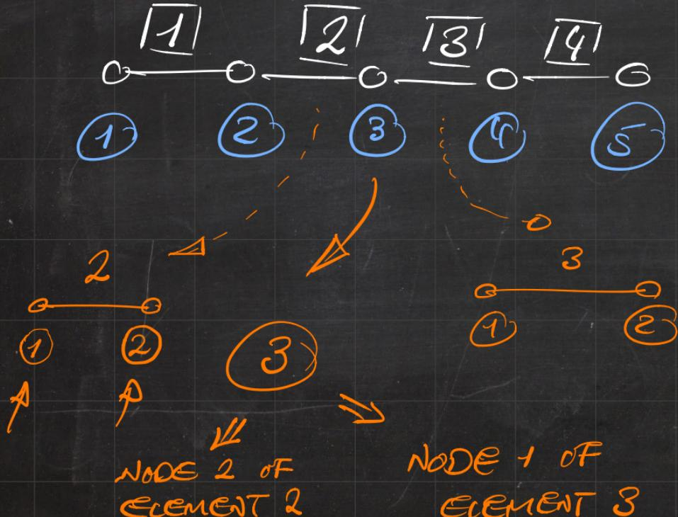
$$\begin{aligned} & \text{Element 2: } k_1 + k_2 \\ & \text{Element 3: } k_1 \\ & \text{Global Structure: } \frac{k_1 + k_2}{k_1 + k_2} \\ & \Rightarrow K = K_2 + K_1 \end{aligned}$$
