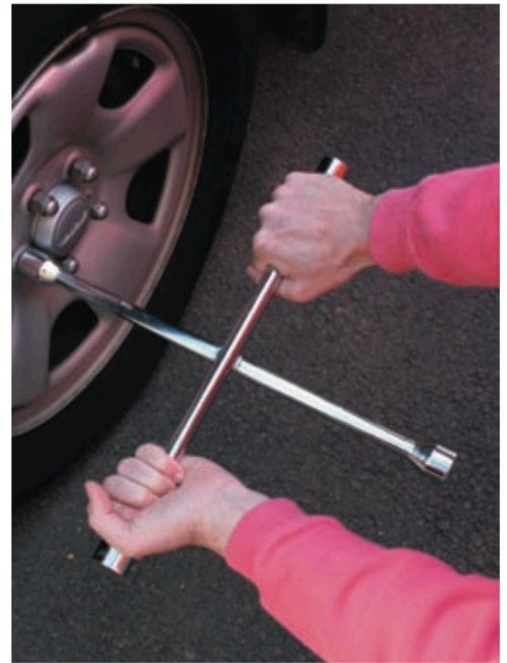
Photo 3.1 The parallel upward and downward forces of equal magnitude exerted on the arms of the lug nut wrench are an example of a couple.
